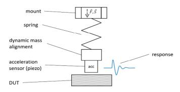
The measurement velocity is adjustable from 0,1 to 60 mm/s to optimize the needed time for measurements or to emulate the movement of real operation. Furthermore, the system is able to record the force that is applied by the finger with an additional high-precision force sensor. Hereby the system can detect the actuating force to trigger haptic feedback.
