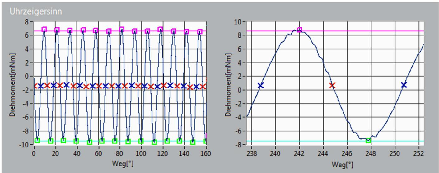
The DTN 38 can be used to verify the suitability of the rotary haptic module DHM as a measuring system in accordance with the guidelines on "Capability certification of measuring systems". (tolerance range  $T \geq \pm 5.00$  mNm; cgk value  $\geq 2.00$ )
